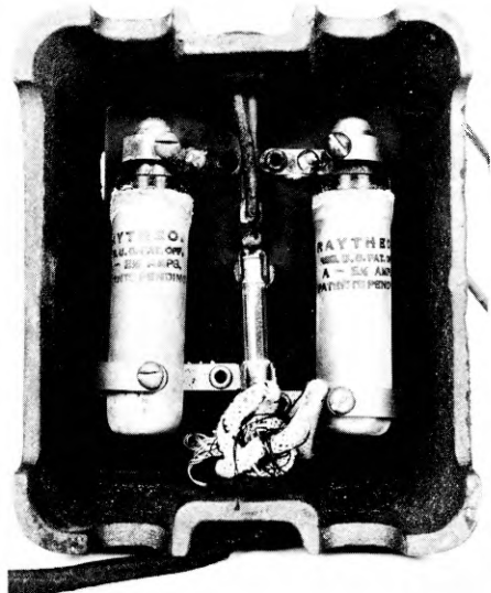
Closeup of Type "A" rectifier.
