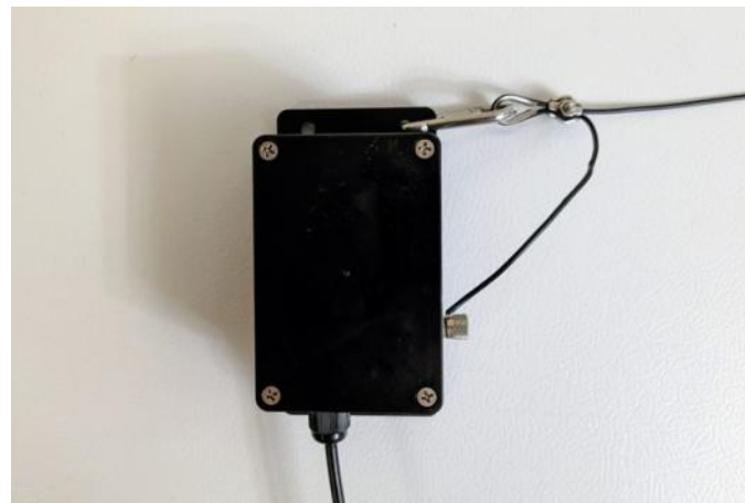
Figure 1: Evil Lair's matching transformer
