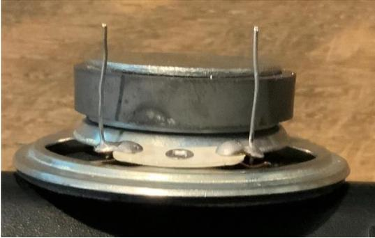
Solder 2 resistor leads to the speaker. Then you can plug the speaker into the breadboard and it will sit on top.
