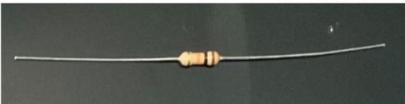
1/4W resistors are a good source of jumpers for use on the breadboard, lead diameter of about 0.02". Cut the leads off at the body of the resistor. That is a perfect length.
